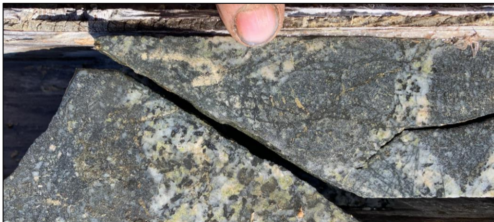
MOF2 - 5.9m @ 0.18 g/t Au & 0.15% Cu Monzonite porphyry with fracture-fill and disseminated chalcopyrite and pyrite
