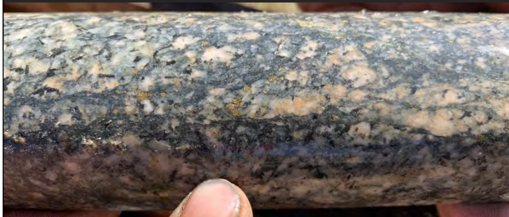
MOF2 - 5.9m @ 0.18 g/t Au & 0.15% Cu Monzonite porphyry with fracture-fill and disseminated chalcopyrite and pyrite
