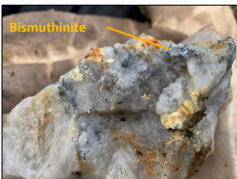
INTRUSION RELATED MINERALIZATION Bismuthinite mineralization in quartz-vein hosted within the Sheldon Stock
